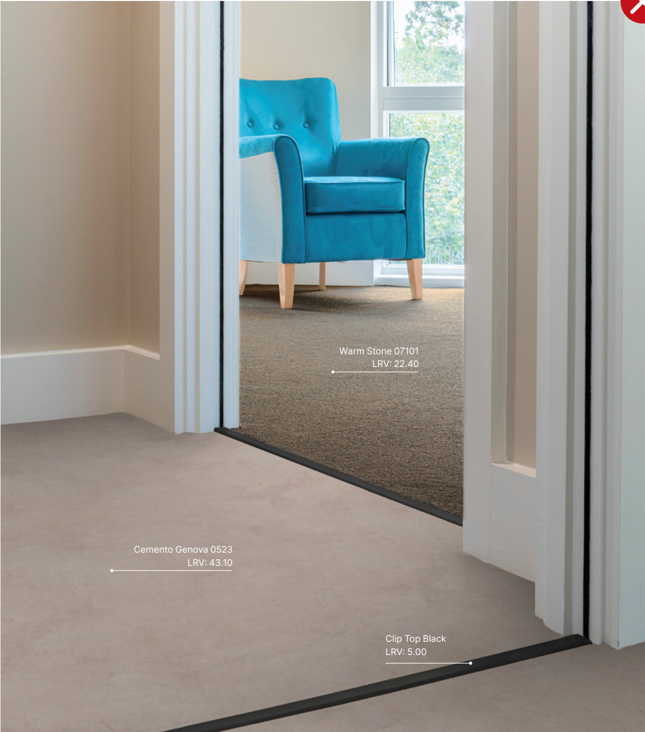
Image shows greater than 10 LRV points between floors, and greater than 3 LRV points between the floor and trim
